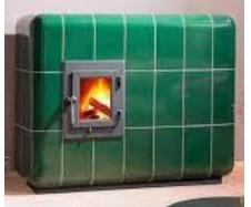
popularity of the *Kachelofen* is based in its efficiency as a home heating source. A small amount of wood is required to provide continuous radiant heat for an entire evening. These masonry headers have extremely high (95%) wood burning combustion efficiencies. Heat transfer efficiency falls within the range of 80 to 85%. This is considerably higher than the efficiency of metal stoves and fireplaces. The enclosed fire box eliminates the danger of smoke and sparks.
