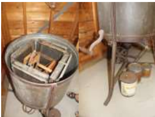
Extractor interior and detail of the turning mechanism.
